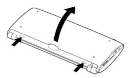
2. Orient the contacts as shown, and then insert the battery pack.
